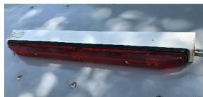
Drill a hole in one side of the square tube to pass the wires through then mount the light bar to the square tube with Gorilla Heavy Duty Double Sided Mounting Tape (Amazon, Home Depot)
